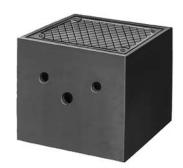
Solid box types for bridge and street lighting. Suitable for underground electrical work. Standard boxes furnished with neoprene gaskets and stainless steel cap screws. Cored or tapped holes for conduit not furnished as standard, available if specified at additional cost – send details showing sizes and locations. Units are shipped assembled.
